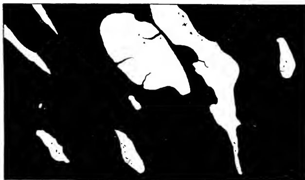
Fig. 41—Character of ore at Levack mine, Sudbury area, Ontario, first level. Black represents sulphides; white represents granite-gneiss. Width of face 3 feet.
